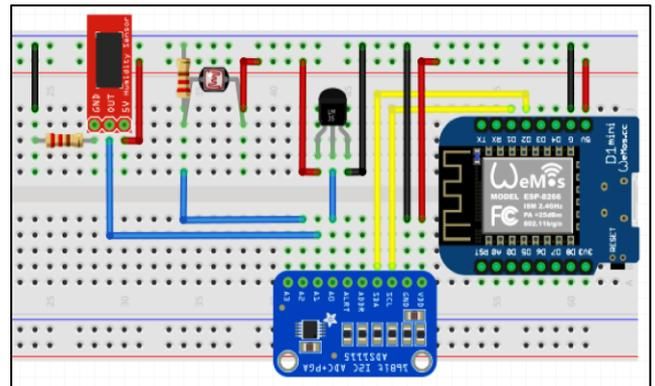
Fig. 8. Circuit design of the weather monitoring hub
