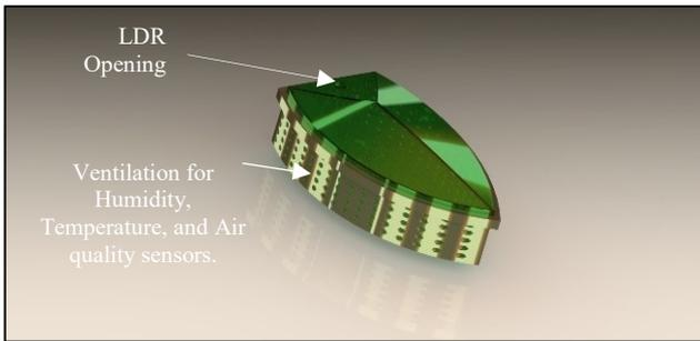
Fig. 9. Design of the weather monitoring hub case
