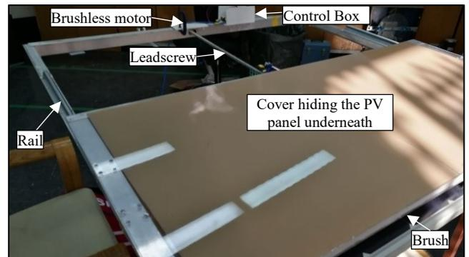
Fig. 17. ASPCS constructed prototype
