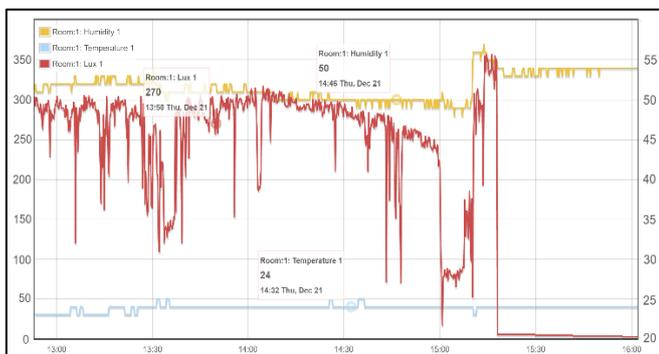
Fig. 15. Example of temperature, humidity (scale on right) and lux (scale on left) readings over a period of time (3 hours)
