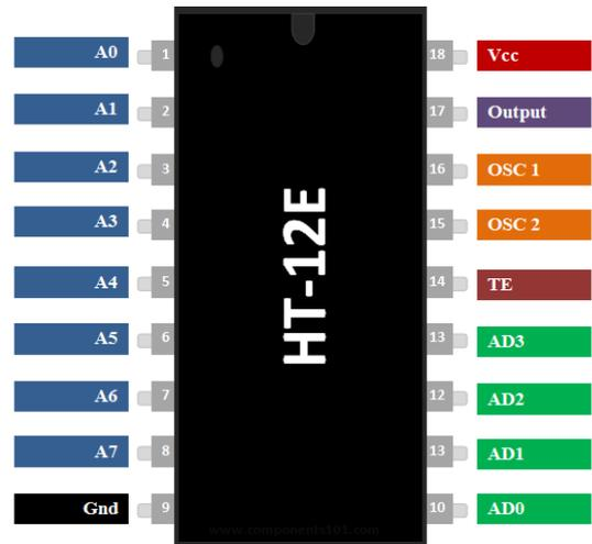
Fig. 3. Pin diagram of HT12E Encoder IC
