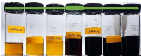
Fig. 3. Shows the degradation of oil sample after predefined interval of distance run by engine.
