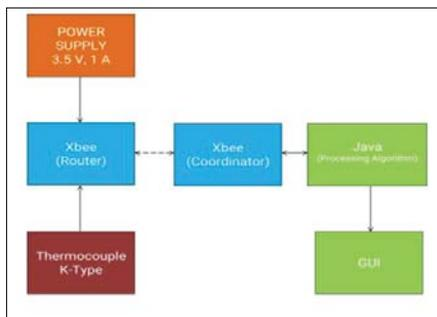
Fig.1. Block Diagram for Wireless Sensor Network Using Xbee, K-type Thermocouple and Java
