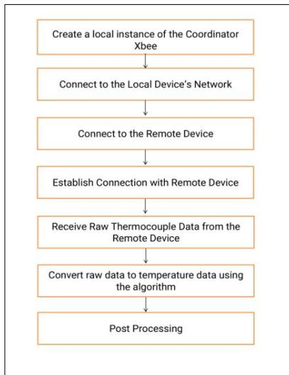
Fig.2. Flow Chart for operation of the Java program
