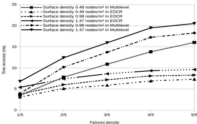
Fig. 6. The time costs of the failures recovery depending on of the failures density and the surface density in Multilevel and EDCR
