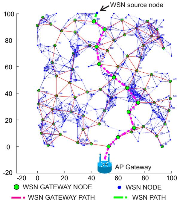
Fig. 3. 1-layer WSN network simulation example (300 WSN nodes).
