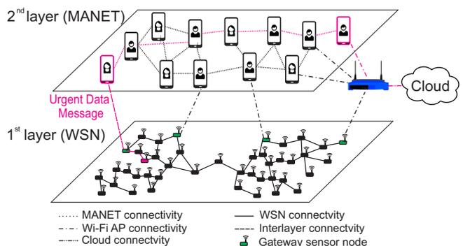
Fig. 2. Proposed 2-Layer network hierarchy comprising Wi-Fi, MANET and Sensor networks.
