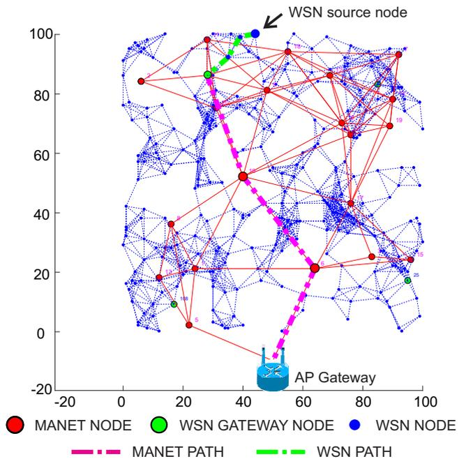
Fig. 4. 2-layer WSN-MANET network simulation example (300 WSN nodes + 20 MANET nodes).
