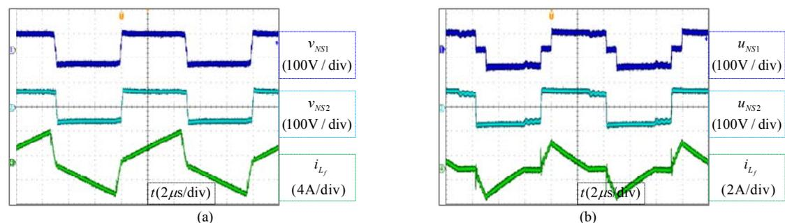
Fig. 16. Experimental waveforms of (a) CCM2 mode, and (b) DCM mode
