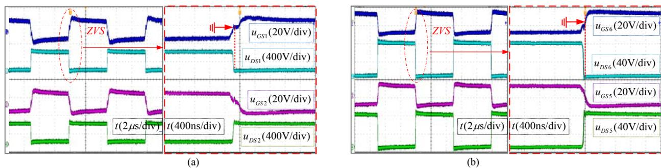
Fig. 17. Switching waveforms of (a) primary-side switches, (b) secondary-side switches.
