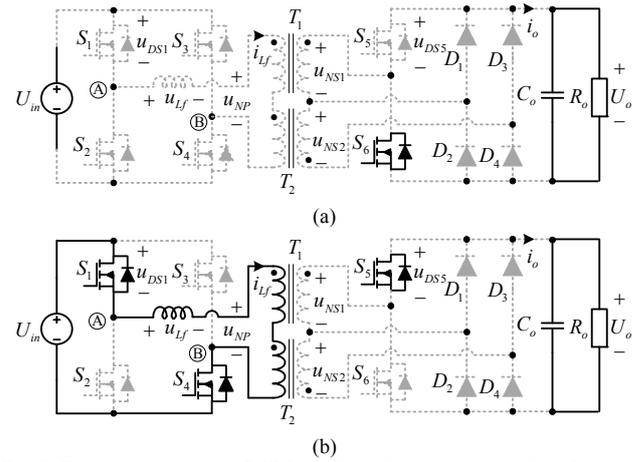
Fig. 8. Equivalent circuits in DCM, (a) Stage 1 [ $t_0, t_1$ ], and (b) Stage 5 [ $t_4, t_5$ ].
