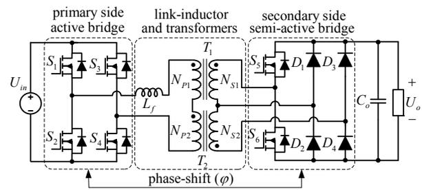
Fig. 1. Topology of the proposed dual-transformer-based asymmetrical dual-bridge converter.
