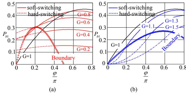
Fig. 11. Soft-switching range of (a) secondary-side switches, and (b) primary-side switches.
