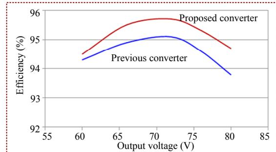
Fig. 23. Efficiency comparison of the proposed converter and previous converter at 1kW output power.
