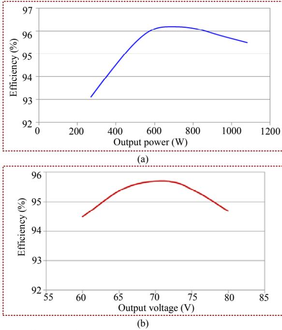
Fig. 19. Efficiency of the proposed DT-ADB converter, (a) at 72V output voltage, (b) at 1kW output power.
