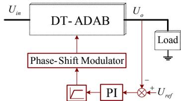
Fig. 12. Control block diagram.
