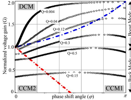
Fig. 9. Output characteristics, (a) normalized output power, (b) normalized voltage gain.
