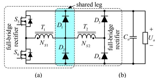
Fig. 2. Secondary side circuit of the DT-ADB converter.
