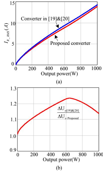
Fig. 21. Comparison of (a) root-mean-square value of rectified current, (b) voltage ripple of output capacitor.
