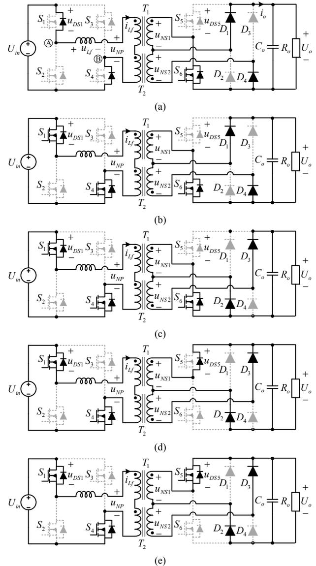
Fig. 4. Equivalent circuits in CCM1, (a) Stage 1 [ $t_0, t_1$ ], (b) Stage 2 [ $t_1, t_2$ ], (c) Stage 3 [ $t_2, t_3$ ], (d) Stage 4 [ $t_3, t_4$ ] and (e) Stage 5 [ $t_4, t_5$ ].
