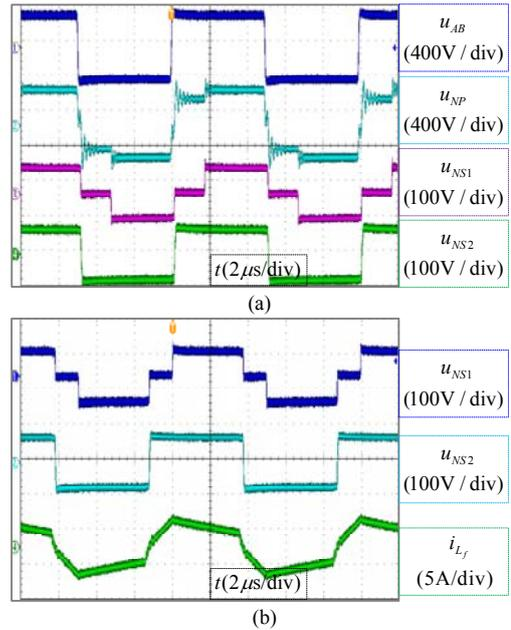
Fig. 14. Experimental waveforms at 80V and 1000W output, (a) waveforms of  $u_{AB}$  (voltage of middle-points of primary side bridge),  $u_{NP}$  (total voltage on primary winding s of the two transformers),  $u_{NS1}$  (voltage of secondary winding of  $T_1$ ) and  $u_{NS2}$  (voltage of secondary winding of  $T_2$ ), (b)  $u_{NS1}$ ,  $u_{NS2}$  and  $i_{L_f}$  (current through the high-frequency-link inductor  $L_f$ ).
