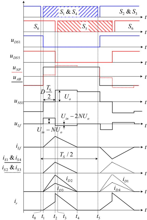
Fig. 7. Waveforms of DCM mode.
