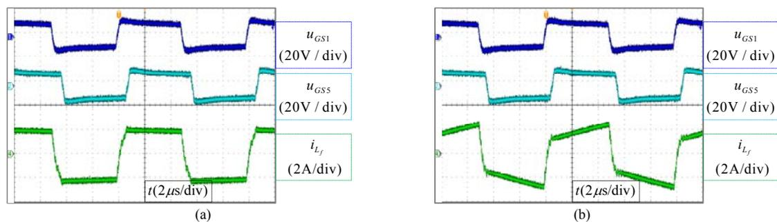
Fig. 15. Experimental waveforms of  $u_{GS1}$  (driving voltage of  $S_1$ ),  $u_{GS5}$  (driving voltage of  $S_5$ ) and  $i_{L_f}$ , (a) balance mode (b) buck mode.
