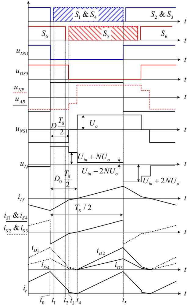
Fig. 5. Waveforms of CCM2 mode.
