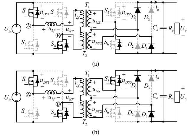
Fig. 6. Equivalent circuits in CCM2, (a) Stage 3 [ $t_2, t_3$ ] and (b) Stage 4 [ $t_3, t_4$ ].
