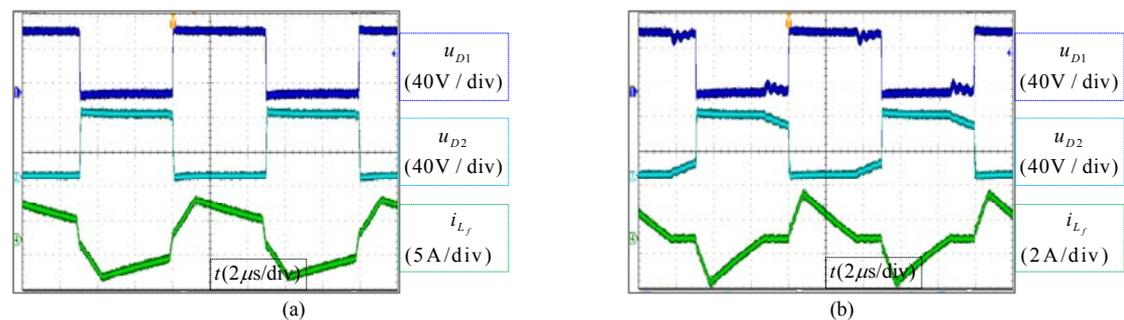
Fig. 18. Switching waveforms of secondary-side diodes, (a) CCM1, (b) DCM.
