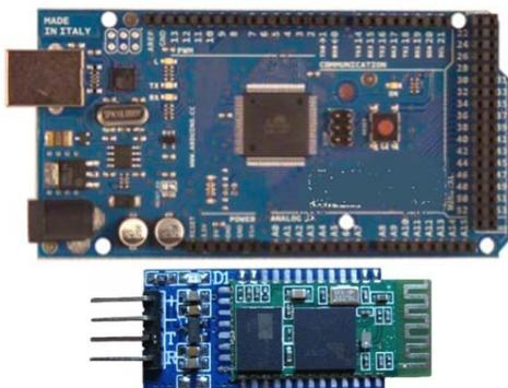
**Fig. 5.** This Figure presents a picture of the development board and its Bluetooth daughter board.
