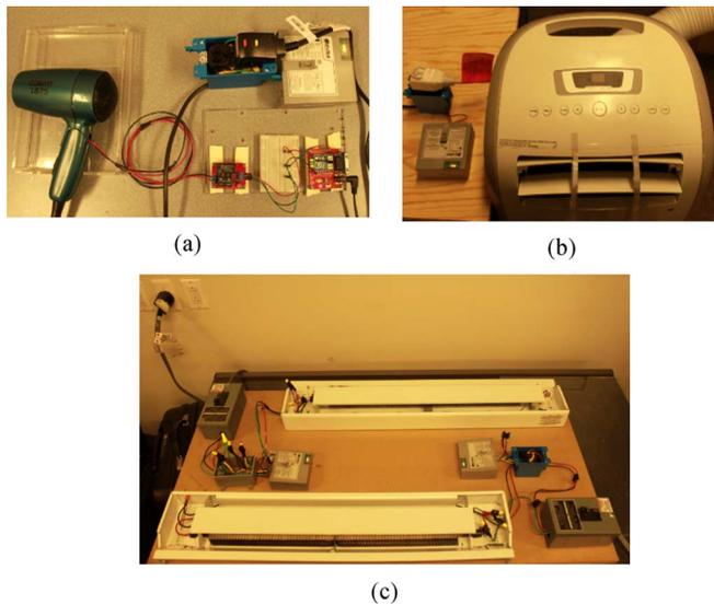
Fig. 2. HEM system installation: (a) a load controller connected to a hair dryer w/ the added relay circuit to allow turning OFF its heating coils; (b) a portable AC unit connected to a load controller; and (c) two sets of a load controller, each connected to an electric baseboard heater.
