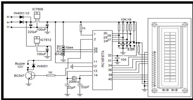
Figure 6 Schematic LCD Display Interface with PIC Microcontroller
