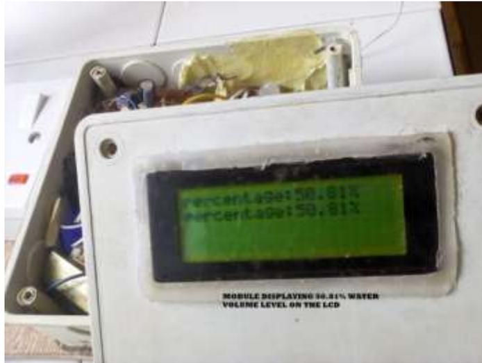
**Figure 7** 50.81% of Volume displayed as output on the LCD
