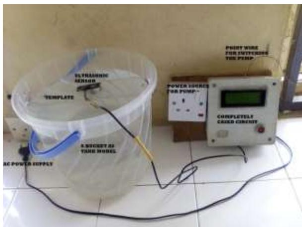
**Fig. 5: Shows the system ready for System Calibration**
