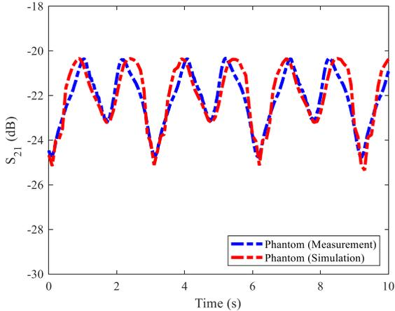
Fig. 5. Normalized  $S_{21}$  vs time for a single arm swing motion at 433MHz for the antenna on both wrists (front) configuration. The plot shows a comparison of data from phantom model measurement and phantom model simulation.
