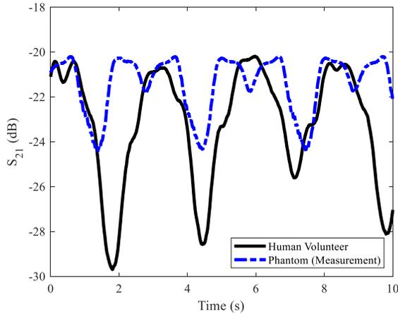
Fig. 4. Normalized  $S_{21}$  vs time for a single arm swing motion at 433MHz for the antenna on chest/left wrist (front) configuration. The plot shows a comparison of data from human volunteer measurement and phantom model measurement.
