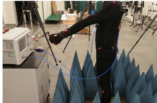
Fig. 3. A human volunteer performing an arm-swinging motion while wearing a motion capture bodysuit and monopole antennas and surrounded by ground absorbers.
