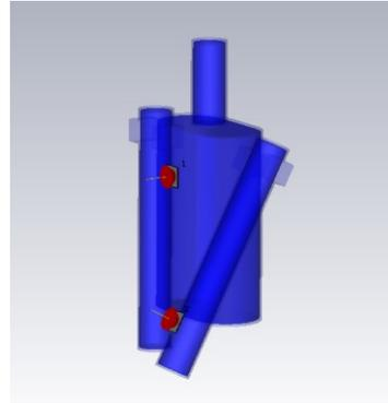
Fig. 2. Human body phantom model in CST with monopole antennas on the chest and left wrist (front).
