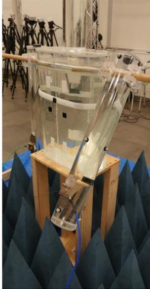
Fig. 1. The phantom model of the human body performing an arm-swinging motion, while having motion capture markers and monopole antennas attached and surrounded by ground absorbers.
