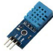
Fig. 3. DHT11 Temperature and Humidity Sensor
