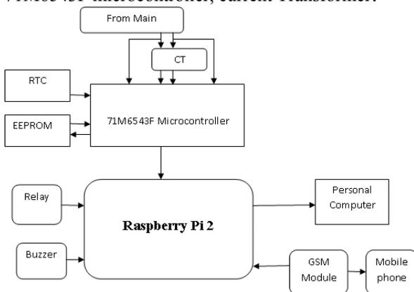
**Fig 1:** Block diagram of pre-paid energy meter.
