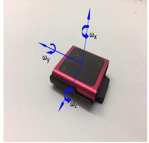
Fig. 3. Tri-axial gyroscope for the experimental setup.
