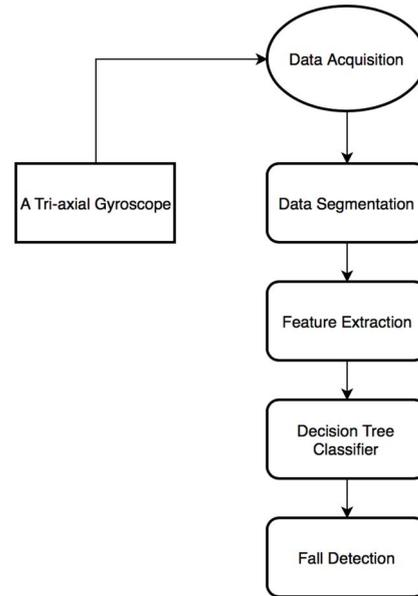
Fig. 1. The workflow of our proposed method
