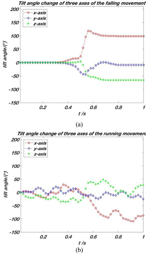
Fig. 4. Tilt angle change of three axes of two different movements: (a) falling, (b) running
